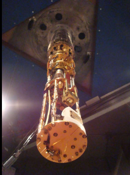
Custom Designed Ultra-low-vibration Dilution Refrigerator
